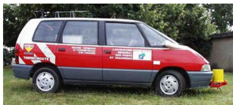
Fig. 1. : Vehicle for thermal mapping
